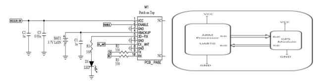
Figure 9. UART interface with ARM
