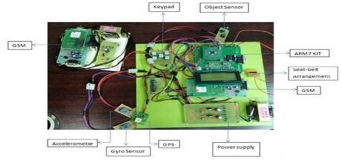
Figure 3. Implementation of Event Data Recorder (Second System)
